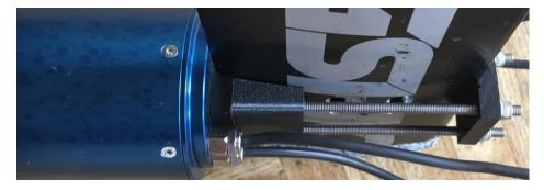
Front and backside are identical spacers, which are catched by M5 screw rods and closed by M5 nuts.
