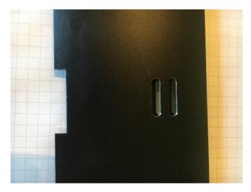
Cut out at end of profile is 8 x 40 mm (depth x height), center is approximately 90-120mm from bottom of profile.
