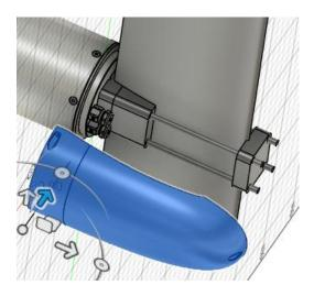
Both cone parts are symmetrical and can be screwed directly on the Mast via M2 screws
